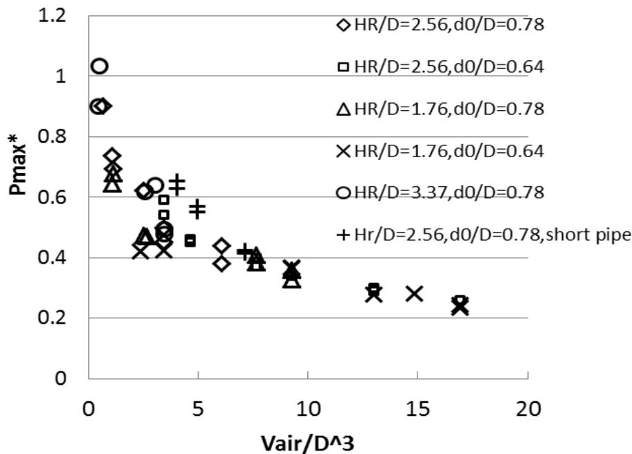
Figure 8: Measured maximum pressures for various experimental configurations and air volumes.
