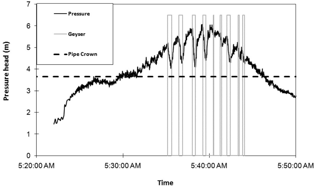
Figure 2: Title of pressure measurement during geyser episode in Minneapolis, Minnesota stormwater system. Gray lines depict the times during which geysers are visible on videotape (no scale). Dashed line depicts pipe crown, flow is surcharged when pressure is above pipe crown.
