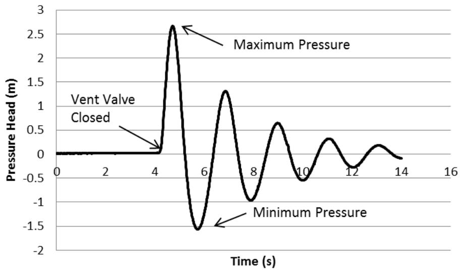
Figure 7: Typical pressure transient.
