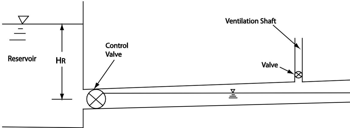
Figure 6: Schematic of experimental apparatus to measure pressure transients due to air compression against an advancing hydraulic bore.
